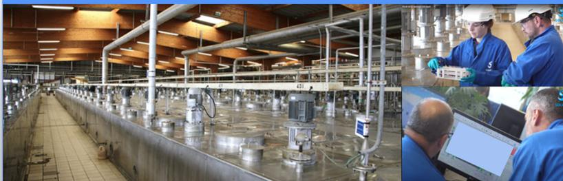
Separation of 2RE requires a "battery" of liquid-liquid extraction devices
