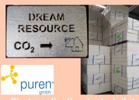
First application tests (pilot status) on foaming plant resulted in CO<sub>2</sub>-based insulation boards @puren gmbh
