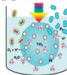
Suspended nanoparticles reactor
