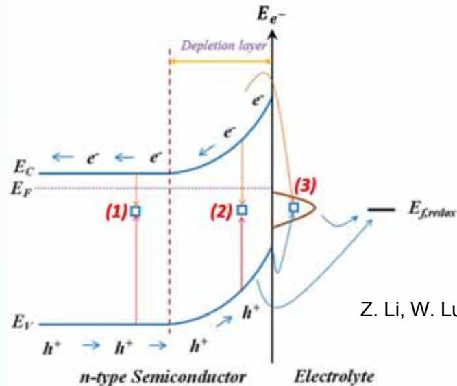
Recombinations in the bulk, inside of the depletion layer or on the surface
