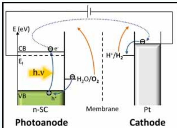
Photoelectrochemical cell (PEC)
